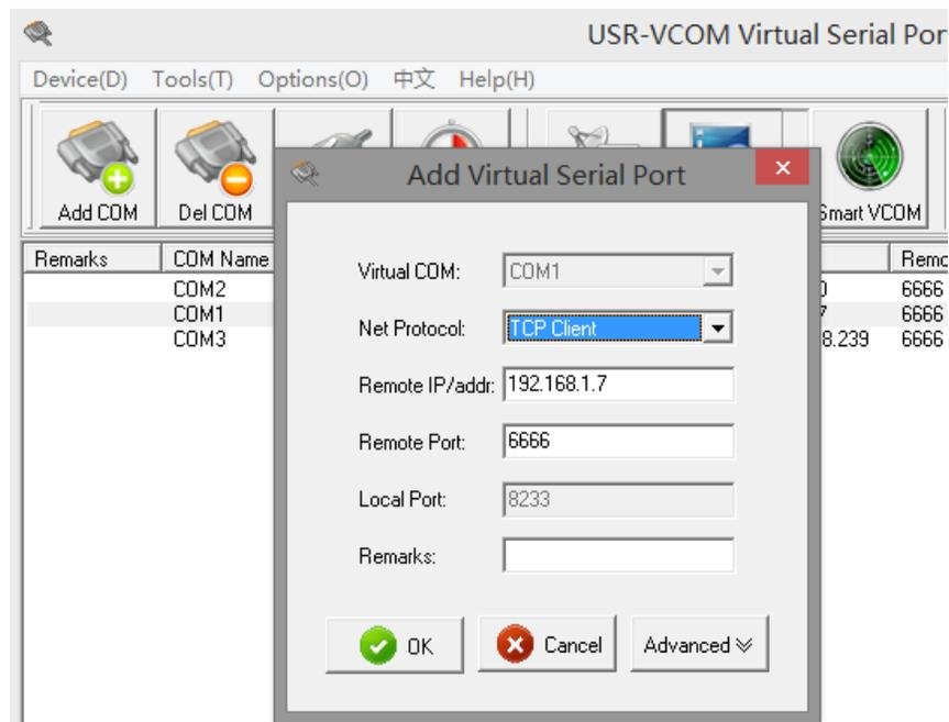
Click OK to add the TCP link. You will see the COM1 will setup at your VCOM, if USB2RJ45 is connect to the router and setting well, the TCP link will be setup, the Net state will shown the connected.
