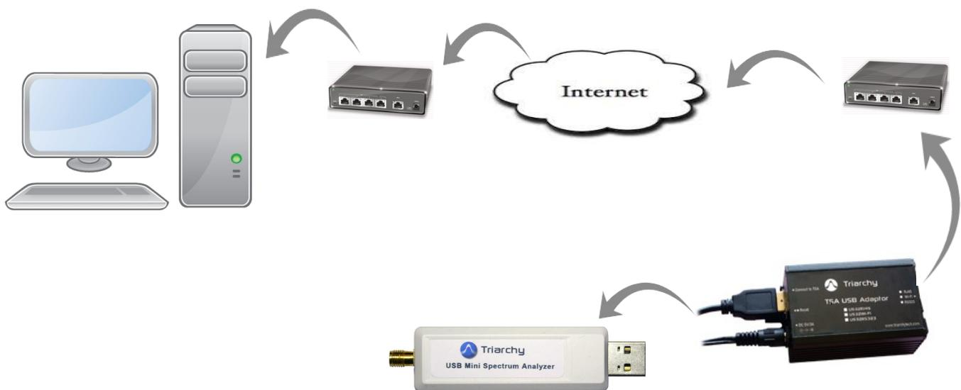
The TSA USB mini spectrum will connect to the USB2RJ45, USB2RJ45 will connect to Router. 5V power supply connects to the USB2RJ45 to provide power.
