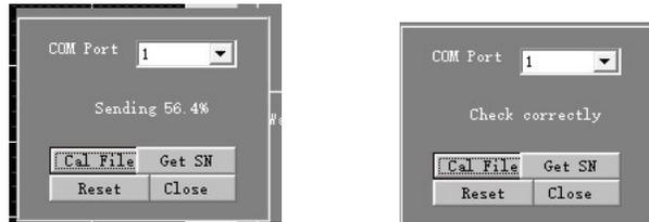
After transfer the calibration file, you can click the Get SN. It means to setup connection with far end TSA dongle. If the communication is successful, the TSA program will shown Device Model TSA6G1 name and Remote connect
